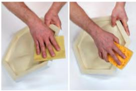
Prepare the ARSTYL® WALL TILES, lightly sand edges if necessary with sandpaper grit 150 or finer (breaks). Wipe edges and panel surface with a damp sponge and dry.
